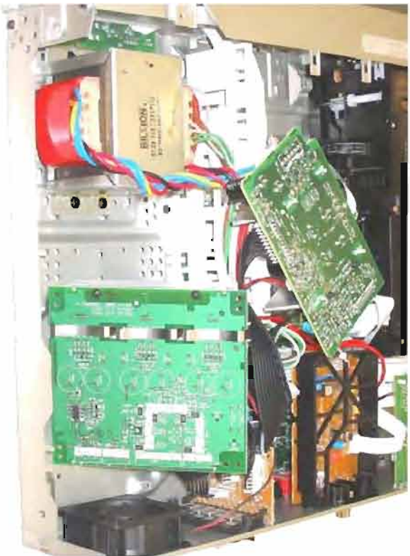
Service position C (Supply and Amplifier boards loose)
